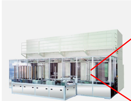
Large Bore Vertical Furnace (VFS-4000, Koyo Thermo Systems Co., Ltd.)
